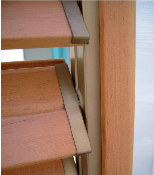
Profiles of anodized or paint coated aluminum, or of galvanized and pre-coated dark brown steel, size 36x14mm, with metal blade holders for housing of slats size 96x14mm, in wood, PVC or aluminum. A pair of galvanized steel bars make up the movement mechanics located inside one of the two profiles.
